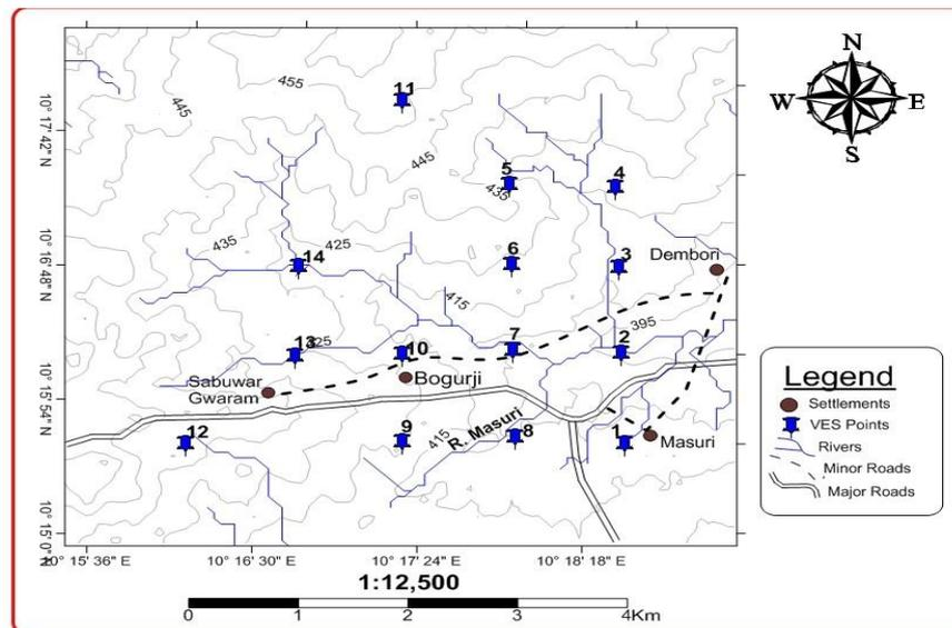
**Fig. 4: Topographic Map of the Area around Masuri Showing the Locations of VES Points**
